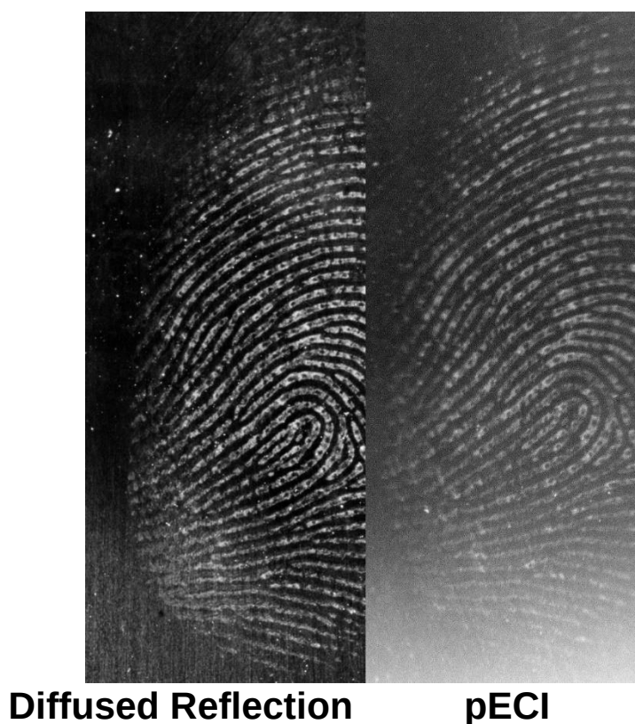
Figure 3.3; Fingerprint impression on glass window enhanced with diffused reflection (left) and pECI v1 (right). pECI Image has black and white inverted to better compare the two image halves. Clear uneven lighting due to uneven flash illumination can be seen in the bottom of the pECI image.
