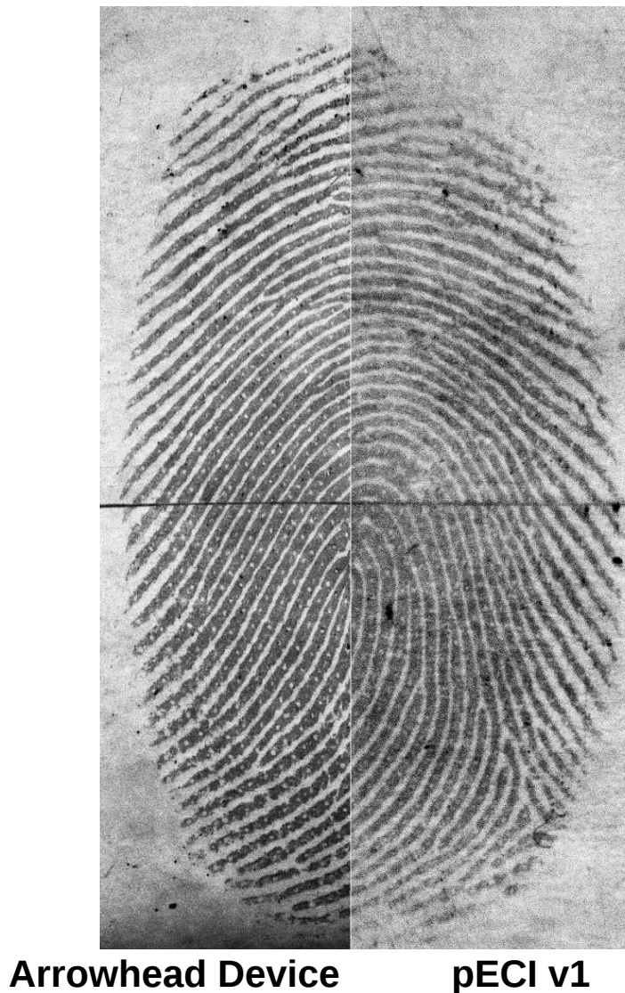
Figure 3.7; A fingermark deposited on a glass substrate enhanced using the Arrowhead device (left) showing more consistent level 3 detail compared to the pECI device (right) with little apparent level 3 features. Both devices were effective in recording level 2 features.
