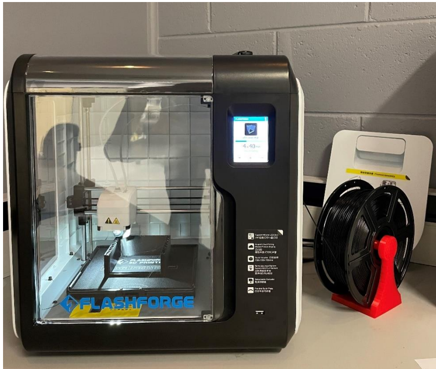
Figure 2.8; Image showing FlashForge adventurer 3D printing new pECI casing.
